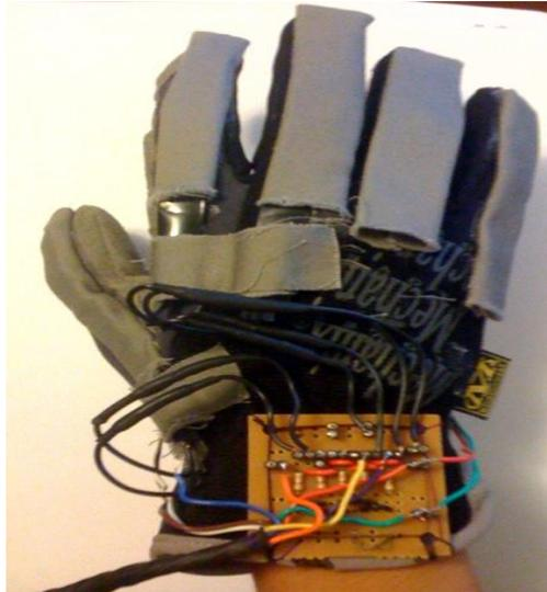
**Fig.3. Photo Shot of our Designed Data Glove**
